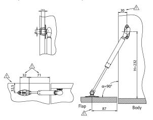
When complying with the relevant fixed dimension  $\triangle$ , an opening angle of  $\alpha = 90^{\circ}$  at an interval of H=232 mm (9.13 in) result.
