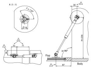
When complying with the relevant fixed dimension  $\triangle$ , an opening angle of  $\alpha = 90^{\circ}$  at an interval of H=236 mm (9.29 in) result.
