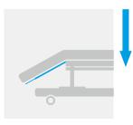
Downwards-movement of the bed-head or the footrest is only possible after using the release lever
