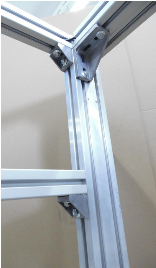
Figure 12 SMS-B-45x90: Examples of connecting the lifting element to the base frame by means of standard connection bracket (small/large)
