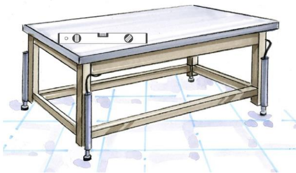
Figure 19 Adjusting the workstation with level
