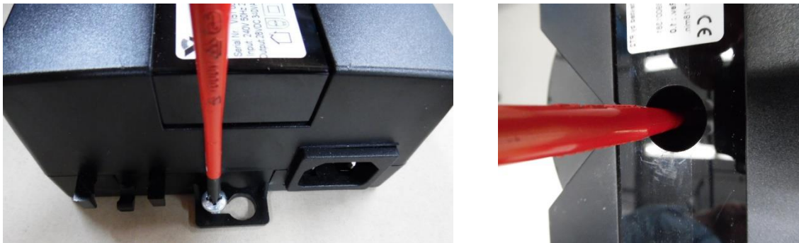
Figure 11 Attaching the electrical controller (screw linkages: left 3x, right 1x)
