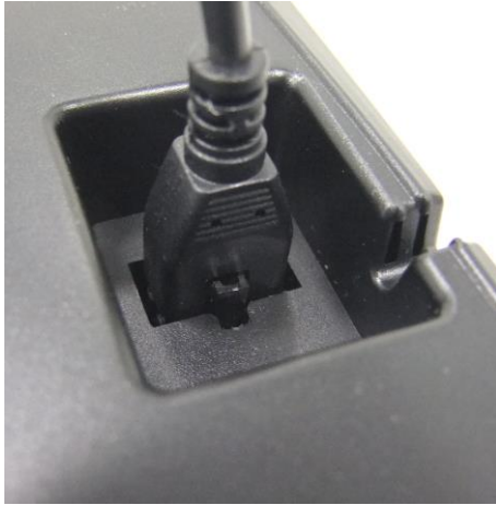
Detailed view of stacking cable connection
