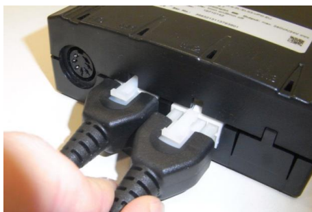
Detailed view of motor cable connection
